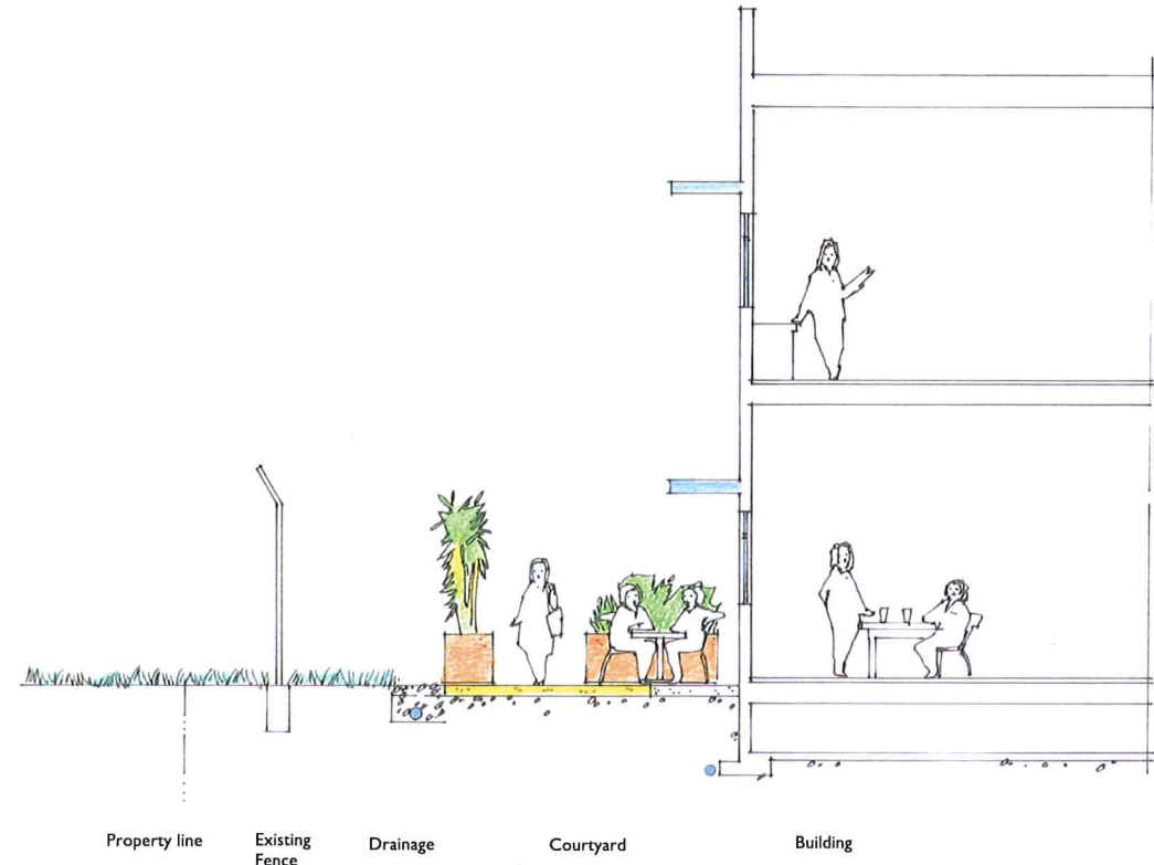
Section C through Courtyard Scale 1:100
